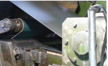
Aluminum sheets are hot and cold coiled at different temperatures to be at different thicknesses. They are used for many industries such as beverage, electrical appliances, office equipments and more.
